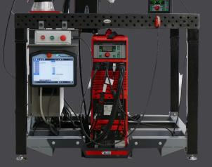
THG Automation has created the URW-2TAPP AC/DC Push-Pull TIG COBOT welding solution for autogenous or wire feed applications. This system is excellent for autogenous welding and has cold wire feed for steel and stainless steel.
